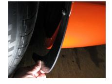
4. Rotate the stone chip guard away from the wheel well lip so that the self-adhesive discs can be seen on the reverse side of the guard. Clean the exposed wheel well lip with alcohol and cotton cloth.
