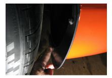
6. Carefully rotate the stone chip guard to the wheel well lip, aligning to your masking tape guide. Once in position, apply pressure to the stone chip guard to adhere the surfaces. Phillips fastener can now be tightened.
