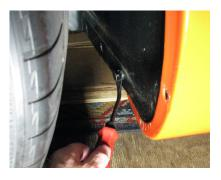
2. Using your flathead screwdriver or trim tool, remove the plastic push-pin fastener from the wheel-well liner. Remove center pin first and then the housing can be removed.
