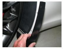
2. Align the upper two  $\frac{1}{4}$ " round holes of the guard with the two open holes of the wheel well lip. Install by re-using the torx fasteners. The cage nuts will move as necessary to line-up with the holes in the stone chip guard and wheel well lip.
