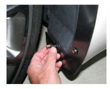
4. The bottom-inner round hole of the guard can now be used to align and drill a ¼" hole in the wheel well shroud. The shroud is made of a composite material and will drill-out easily.
