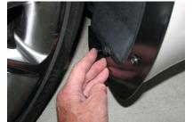
6. Once seated, push the pin into the fastener to lock. Note; The five oval shaped holes at the bottom of the stone chip guard allow air-flow into the sill of the Viper.
